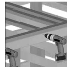
Connect with self-tapping screw (ST02)
