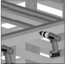
Connect with self-tapping screw (ST02)
