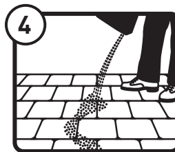
4 Spread more product to fill joints again. Use the street broom again.
